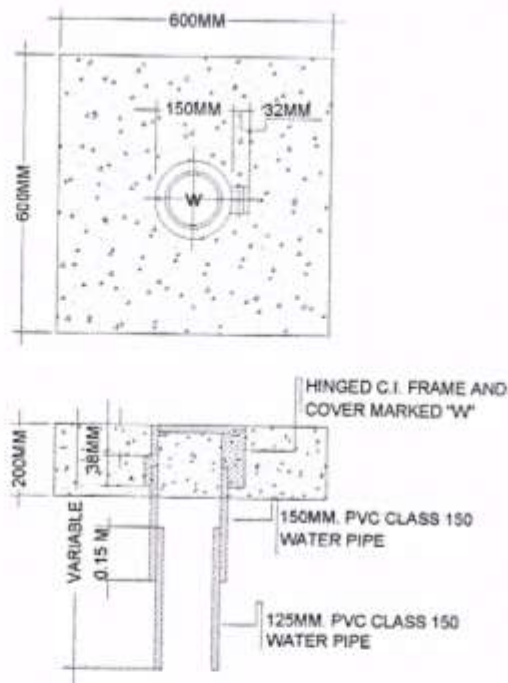
VALVE BOX and COVER DETAIL NOT TO SCALE
