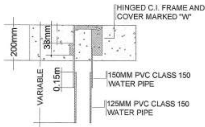
VALVE BOX AND COVER DETAILS
